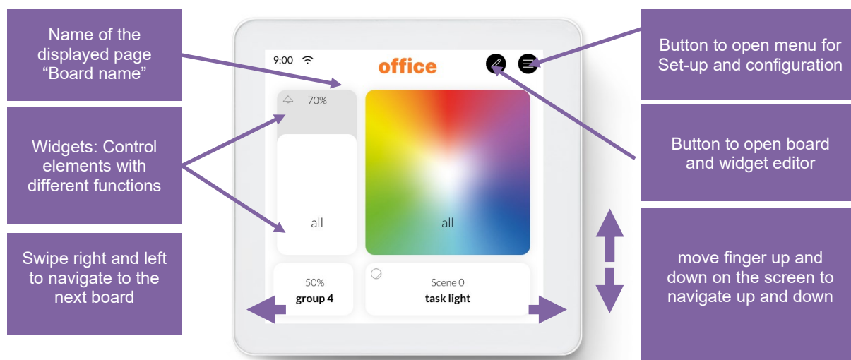
Figure 4 User Interface for Light Control DALI Display 4"
